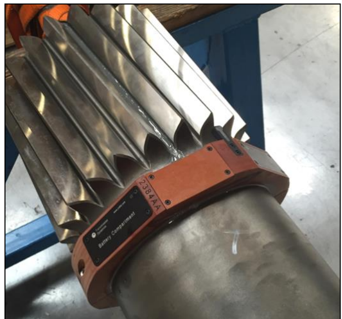
An example of remotely acquired data from double helical gear operating in Wind Turbine application
